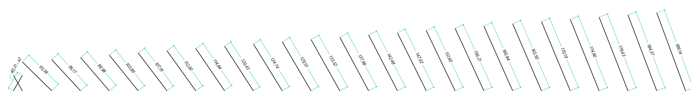
DIAGONAL PERFIL "U" SIMPLIS 127x40#14 3.25Kg/m
